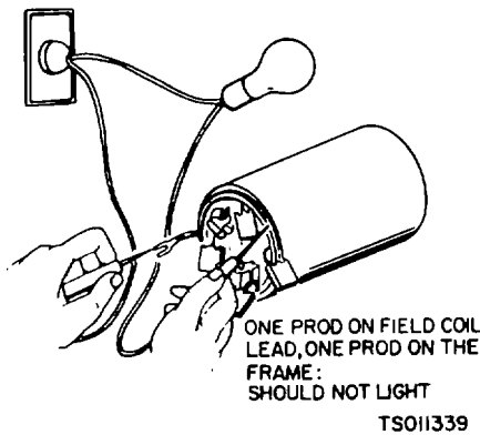
Figure 6-6. Field Coil Ground Test
